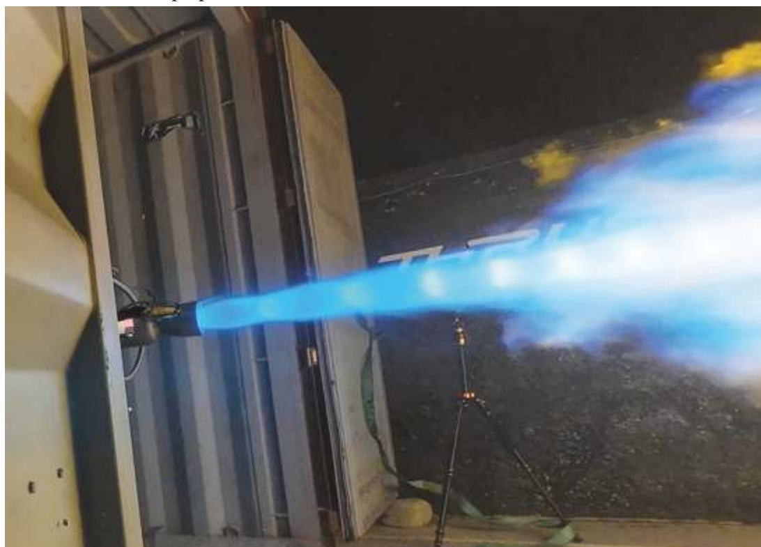
Hotfire of the test combustion chamber
