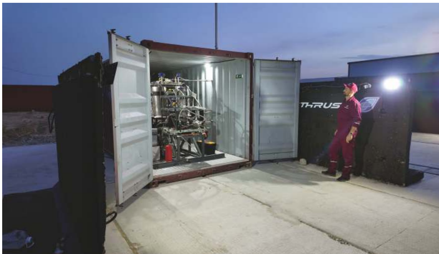
Modular test stand LETS-1.1 for testing liquid propellant rocket engines
